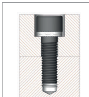
Countersunk socket head bolt secured in position
